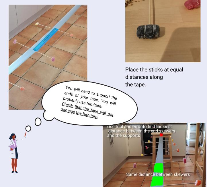
Once you're set up, push down one side of one of the end skewers, let go and watch the wave travel along the tape.
